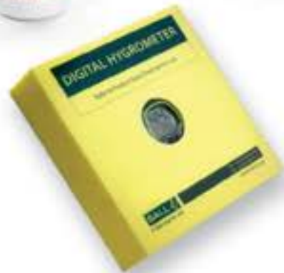
F7346 Digital Hygrometer Box F7346B Butyl Tape To accurately determine the relative humidity of a subfloor. The pre-calibrated hygrometer box incorporates an accurate thermo hygrometer that indicates both relative humidity and air temperature. Uses butyl tape to create airtight seal.
