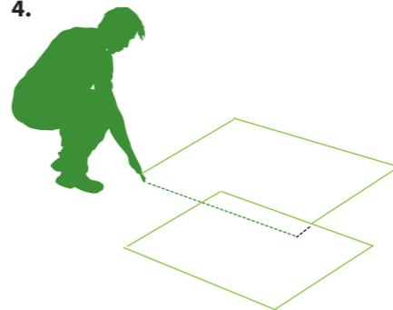
Once complete you can install an additional layer of the weed membrane. This is an extra layer not to be confused with the must have layer between soil and builders' sand. This should be stretched out and fixed using 4" nails around the perimeters and then trimmed.
