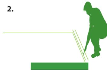
Using a rake level the area off to natural falls as you don't want humps and bumps before installing the stone base. Where there is no edge to butt into, install either a treated timber edge or metal edging. Lay geotextile weed membrane and install a 50mm layer of 6-10mm sharp builders' sand.
