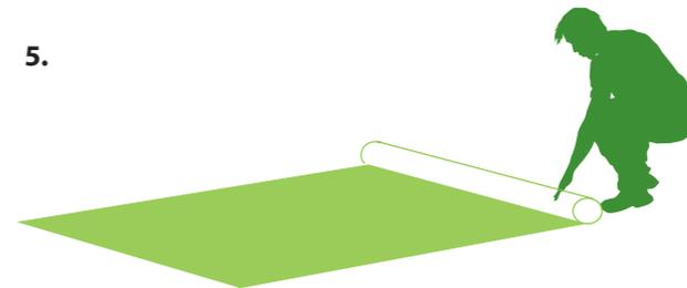
Unroll the grass and position ideally running the pile towards the house on back gardens and the reverse on front lawns (ie facing out). When laying the artificial grass, ensure it fits up to the outer perimeters. Where there is an obstacle like a tree or post fold the grass back and decide the shortest route to cut.
